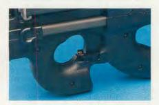
The grip portion of the P90's receiver body has been molded into the configuration of an abbreviated thumbhole stock. The selective-fire dial is directly under the trigger and thus is completely ambidextrous, as are all of the P90's controls. Photo: courtesy FN Herstal
